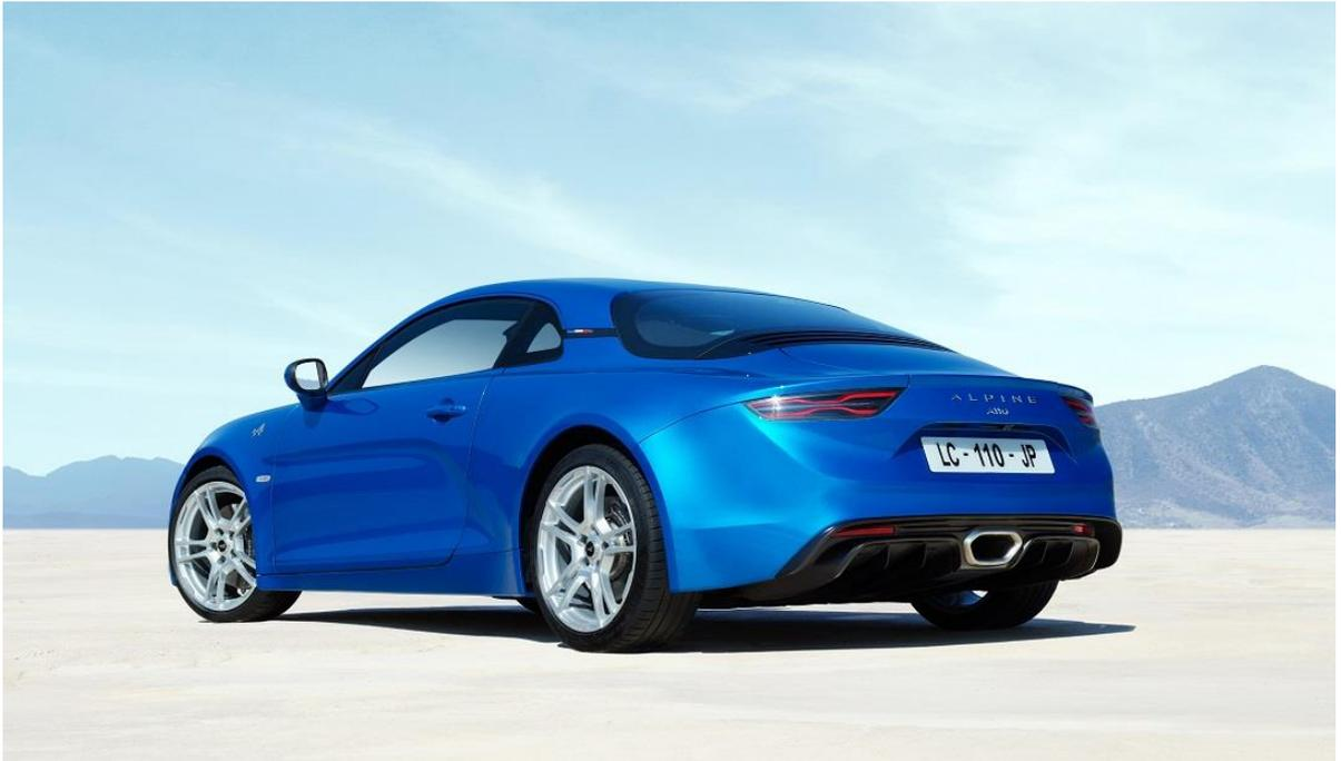
This model has been renamed A110, and its agility and zip are unparalleled: its mass has been optimally spread out (44% at the front, 56% at the rear with the engine in a central-back position) and it is lighter (1,102 kg unladen). It comes with the Alpine chassis and Sport seats, and its efficiency and communicative behaviour in all circumstances provide undiluted driving pleasure.
