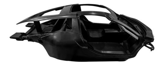
Carbon fibre composite is also used for the crash protection structures that absorb and dissipate impact energy to protect the monocoque at the front and rear. Unusually, the rear subframe is also constructed in carbon fibre and is bolted to the primary chassis structure.
