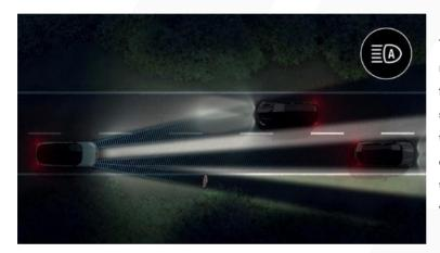
The Matrix LED Vision (Matrix beam / ADB) means drivers can continue using high beam for the greatest coverage no matter what the surrounding traffic is like. This is made possible thanks to anti-glare LED technology that adapts the direction of light beams to ensure the comfort and safety all those in nearby vehicles.
