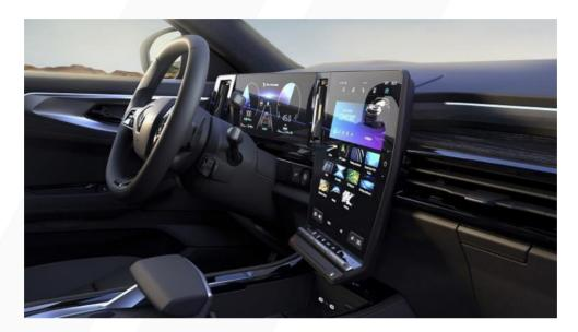
The finish on the OpenR screen has been made to the same standards as high-end tablets and smartphones. The screen is covered in Gorilla-Glass aluminosilicate glass – tempered glass that is ultra-resistant to scratches, everyday bumps, and repeated cleaning. Is has also been given additional anti-fingerprint and anti-glare coatings to keep it is as much a pleasure to touch as it is to see.
