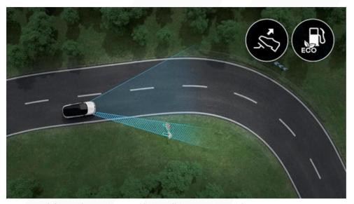
The novel **predictive eco- driving advice** feature is available on the Mild Hybrid automatic versions of the All-New Austral<sup>14</sup>. With an icon that displays on the dashboard or 9.3-inch Head-Up Display, it tells the driver when to ease up on the accelerator to save fuel (and to therefore emit less CO<sub>2</sub>) when approaching a particular road event (sharp
