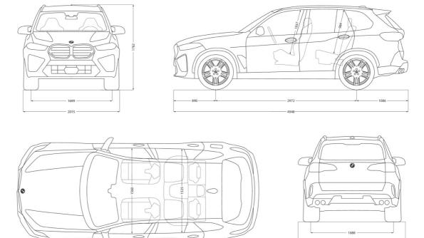
The dimensions indicated in the technical drawing are in millimetres and may vary depending on the model and the items of optional equipment fitted.
